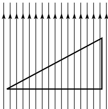
The lower leg of the triangle has width  $w$ , the lower left angle is  $\theta$ , and the length of the prism (in and out of the page) is  $L$ . Verify Gauss's law by direct calculation.
