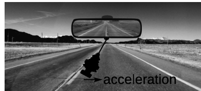
Figure 3.6: The car has just swerved to the right. The air freshener hanging from the rear-view mirror acts as an accelerometer, showing that the acceleration vector is to the right.
